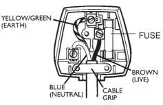
The wire which is coloured BROWN must be connected to the terminal which is marked with the letter L or coloured RED or BROWN.
