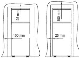
Diagrams show alternative methods of providing correct air flow around the appliance.
