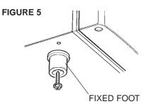
Unscrew the fixed foot and refit it to the hole in the opposite corner of the base of the housing (Figure 5).
