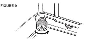
Adjust the adjustable foot to level the appliance (Figure 9).
