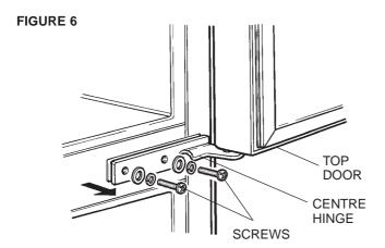
Open the top door and unscrew the screws to remove the centre hinge, spacers and washers. Lift away the top door (Figure 6).
