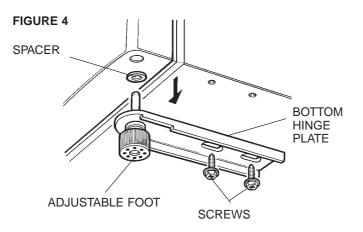
Unscrew the screws to release the bottom hinge plate with adjustable foot (Figure 4).
