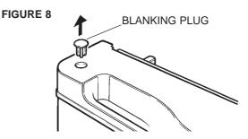
Prise the blanking plug out of its hole in the top edge of the door (Figure 8). Push the plug into the hole in the opposite corner of the top edge of the door.
