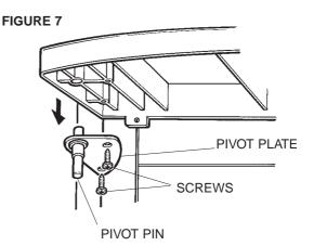
Unscrew the pivot plate from the underside of the cabinet top (Figure 7). Transfer the pivot plate to the mounting holes in the opposite corner of the underside of the cabinet top and fasten it in place.
