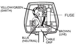
The wire which is coloured BLUE must be connected to the terminal in the plug which is marked with the letter N or coloured BLACK or BLUE.
